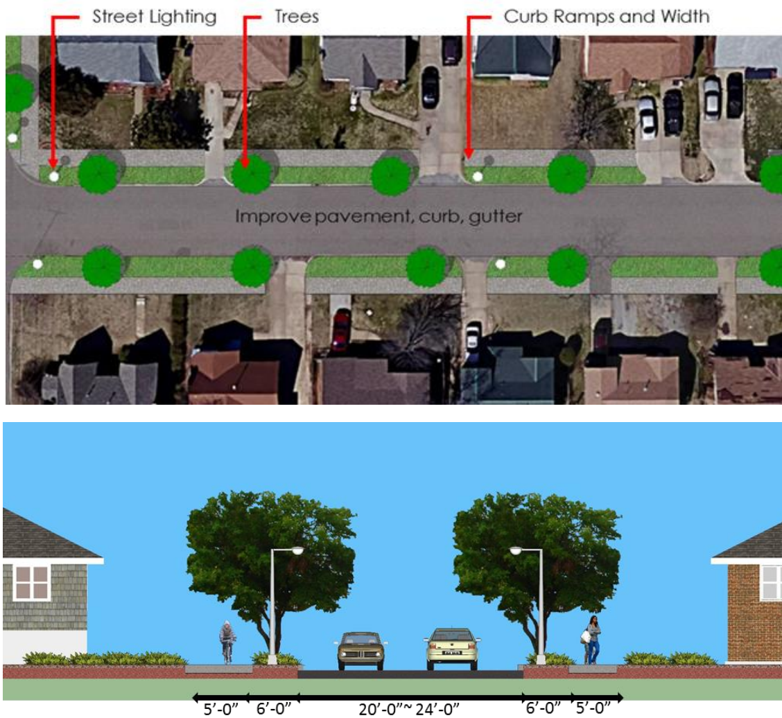
Figure 4.8: Design Examples in NE26th Street for Street Scene Improvement of Residential Collector
